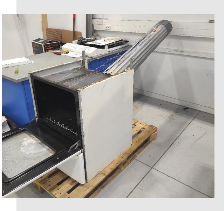
Figure 2. Photograph of the repurposed oven, showing the door opening, sheet metal chimney, and door with the inner glass pane replaced with sheet metal.
